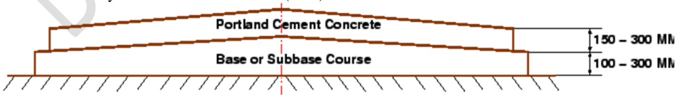
Figure 3: Typical Cross section of rigid pavement
